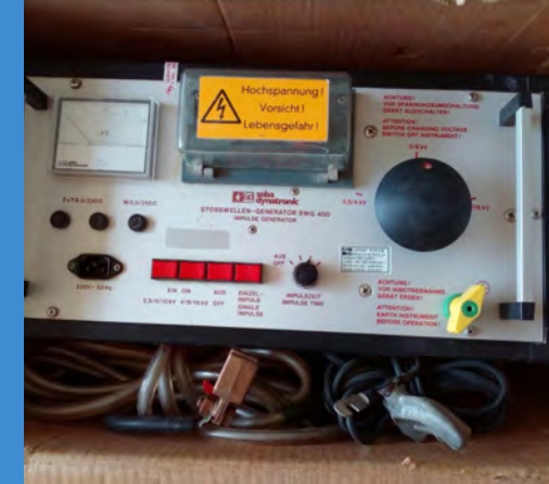
SURGE WAVE GENERATOR
