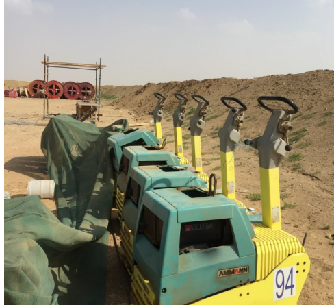
ASPHALT PLATE COMPACTOR
