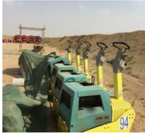
ASPHALT PLATE COMPACTOR
